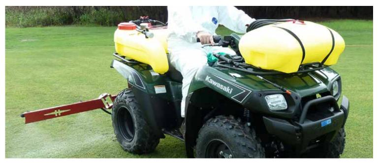
**HARDI ATV Bike** sprayers are made to fit most quad bikes, allowing the bike to become an effective and versatile sprayer with 75 litre on the back and 50L on the front. The bike sprayers are designed to provide a low centre of gravity and the tank shape has smooth contours for easy cleaning.
